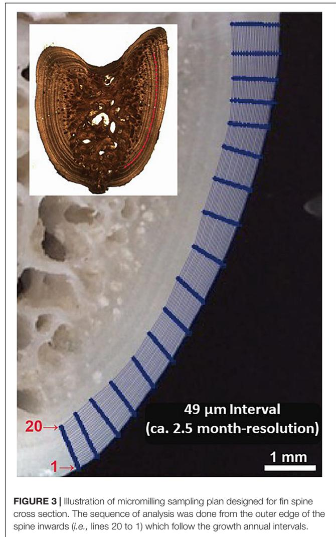
**FIGURE 3** | Illustration of micromilling sampling plan designed for fin spine cross section. The sequence of analysis was done from the outer edge of the spine inwards (i.e., lines 20 to 1) which follow the growth annual intervals.
